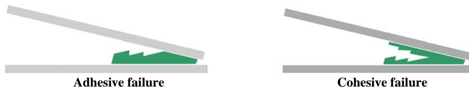
Figure 1: Adhesive and cohesive failure.
